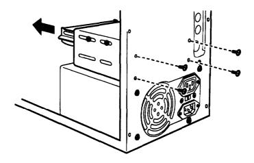
4. Remove the four screws securing the drive to the bracket and slide the drive out of the bracket.
